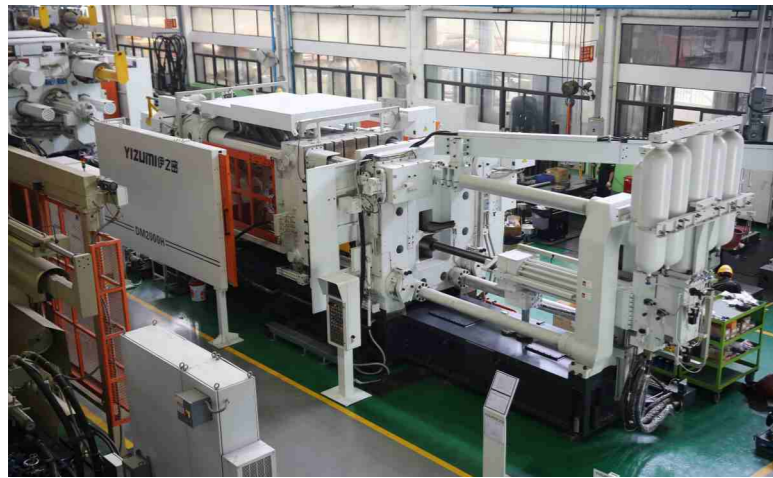
Assembly of 2000H die casting machine completed
