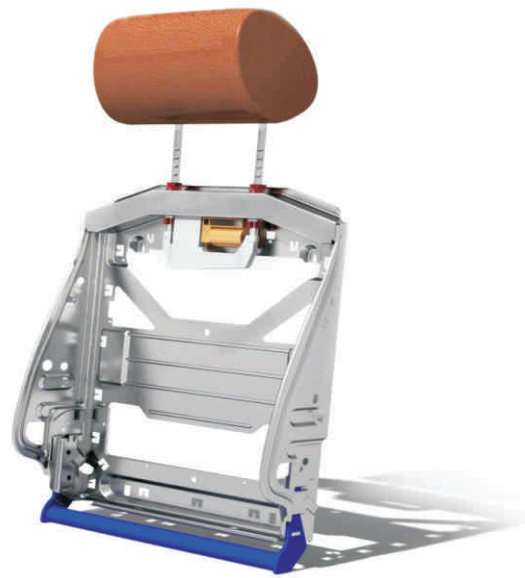
Figure 4: Car seat skeleton construction diagram
