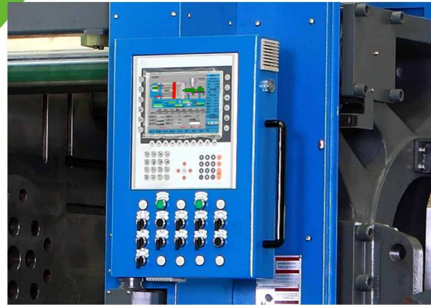
The 10.4-inch touch screen and 500MHz controller facilitate operation and high-speed control via Ethernet.
