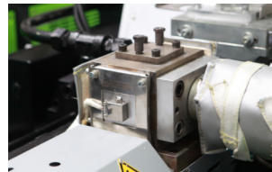
Connecting area between injection molding machine and CDS
